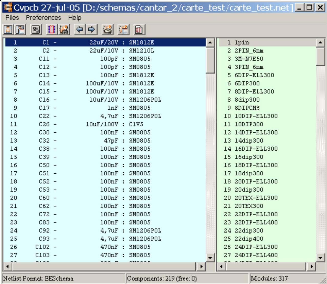
The **Component** window (on the left) displays the list of components appearing in the Netlist read.
