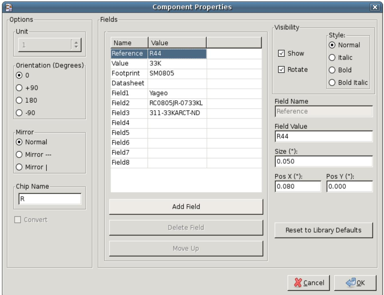
Using the BOM Format **Single Part per line** only requires the Component properties be edited for one Component on the schematic and not all the Components with that same Value.
