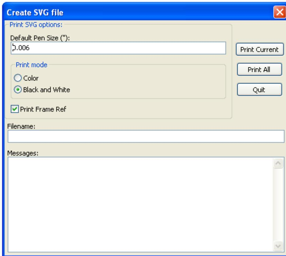
Allows you to create plot files using the vectored format SVG.
