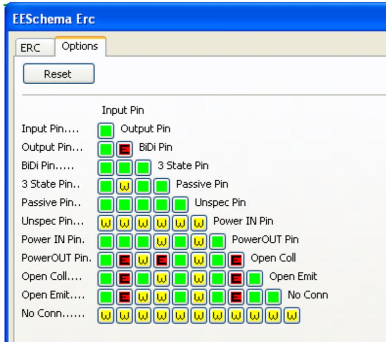
This Setup ERC dialog box allows you to establish connectivity rules between pins; you can choose between 3 options for each case :
