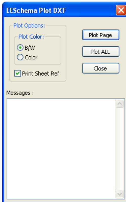
Allows you to create plot files using the format DXF.
