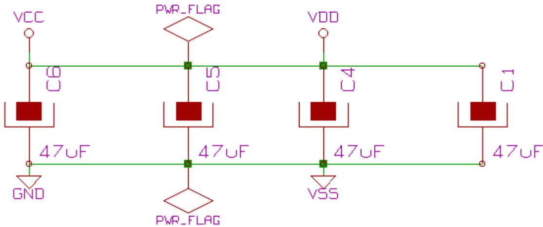
In this example, ground (GND) is connected to power port VSS, and power port VCC is connected to VDD. Two PWR\_FLAG symbols are visible. They indicate that the two power ports VCC and GND are really connected to a power source.
