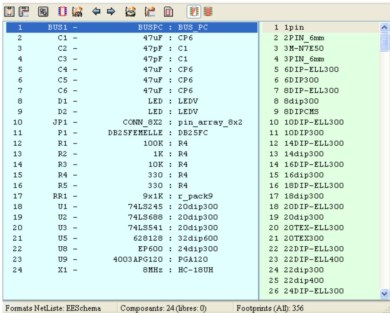
The screenshot shows the Cvpcb component placement tool interface. The main window displays a list of components and their corresponding footprints. The components are listed in a table with columns for component ID, component name, value, and footprint name. The footprint names are listed in a separate column on the right. The status bar at the bottom shows the current format (NetListe: EESchema), the number of components (24), and the number of footprints (356).
