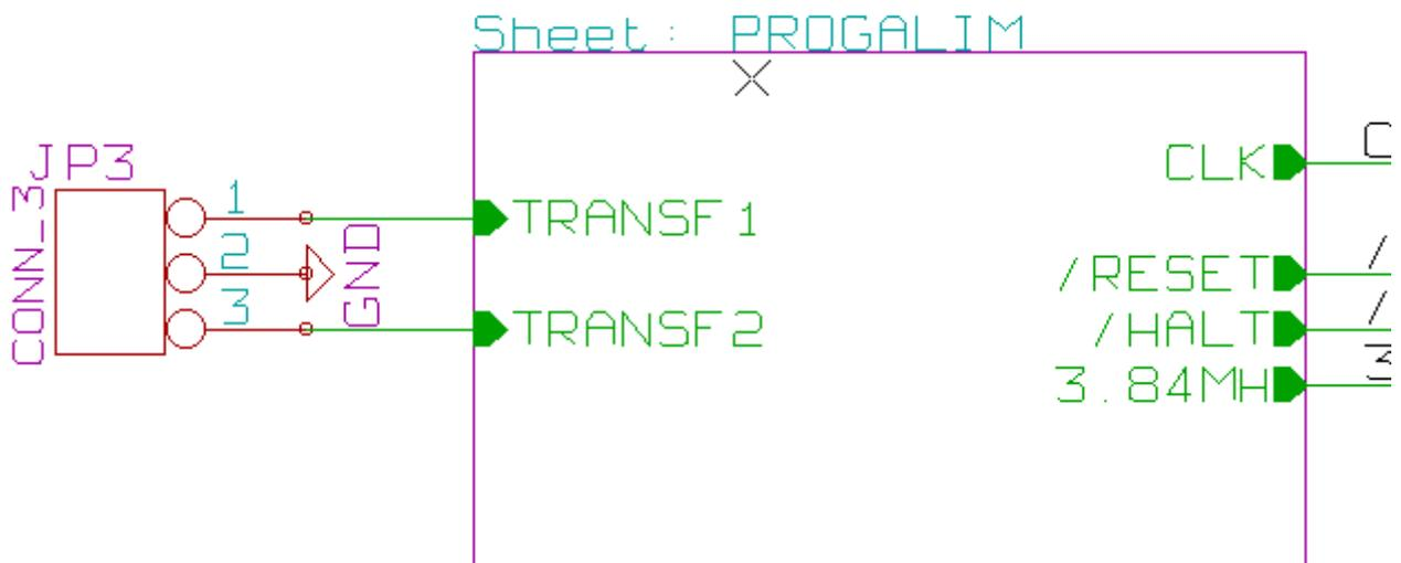
You find again, the two corresponding HLabels, providing connection between the two hierarchical sheets.
