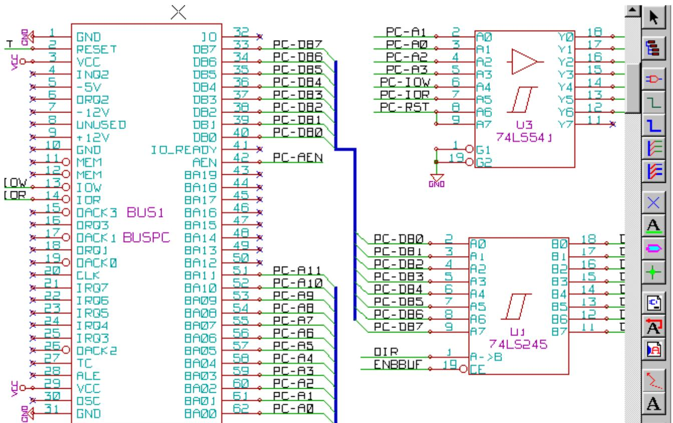
Many pins (particularly component U1 and BUS1) are connected to buses.
